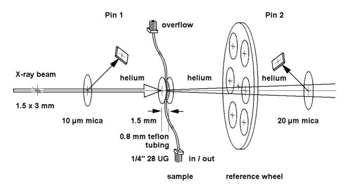
Figure 1: Sample environment for SAXS with protein or polymer solutions in a flat mica flow-through cell.
