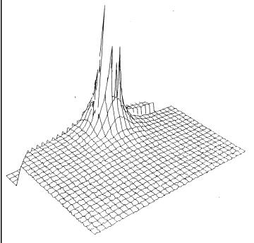
Fig.1: The X-ray small angle scattering of cytochrome-c reductase (cytochrome-bc<sub>1</sub> complex) shows a weak side maximum, which is visible also in the crude data. It results from the Htype structure of the membrane protein.
