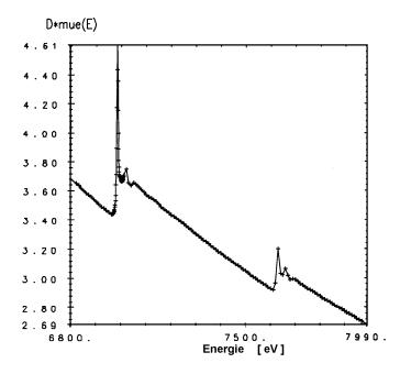
Figure 2: The EXAFS spectrum of 50 mM EuDTPA solution shows the LIII and LII absorption edges while the sample contained only 0.76% metal. The bright white line of the LIII-edge is favourate for structure labeling. The spectrum was estimated at the B1-beamline with a novel flat window flow-through cell (8mm).
