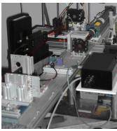
Dynamic Light Scattering device (DLS) at TUM-E17. The modular setup can be equipped with a magnet or stopped-flow device for field and time-resolved experiments. The backscattering setur (170°) enables the investigation of concentrated original samples (5 % w/w)
